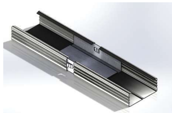
Schematic representation of a CD-60 profile connection with the help of a CD-connector.
